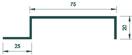
frame Profile Section Sand Trap Louvers
